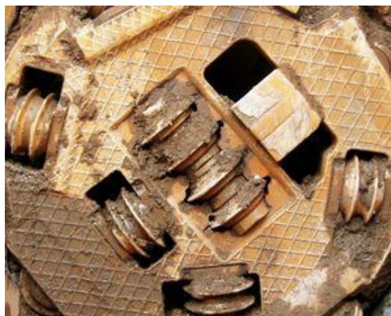
Borehoved for mikrotunneling - slurymaskine
